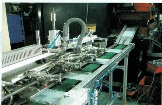
衝壓線上末段成形攻牙作業 ▶ the last stage of forming tapping operation
